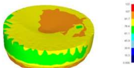
Figure 2.6: Contour Plot of Effective Stress (N-mm 2 ) during rotary Forging.
